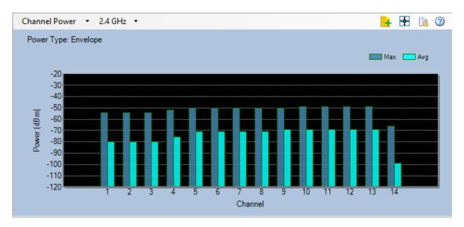
The Channel Power can be defined either as Envelope or Integrated. Envelope power is defined as the maximum, or peak, energy level in a channel's frequency range. Integrated power is similar, and is defined as the average power of all frequency power levels in a channel's frequency range. In the bar chart, the Max bar corresponds to the Max data line on the FFT chart, while the Avg bar corresponds to the Average data line on the FFT graph.
