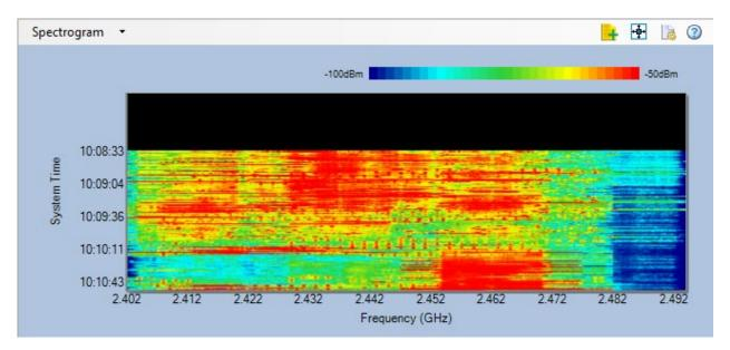
Each time the adapter scans the RF spectrum makes one sweep cycle, which is represented by a horizontal (colored) line across the spectrogram plot. The spectrogram scrolls dynamically upward as the application scans the spectrum. New data appear at the bottom of the graph while old data are constantly pushed to the top.
