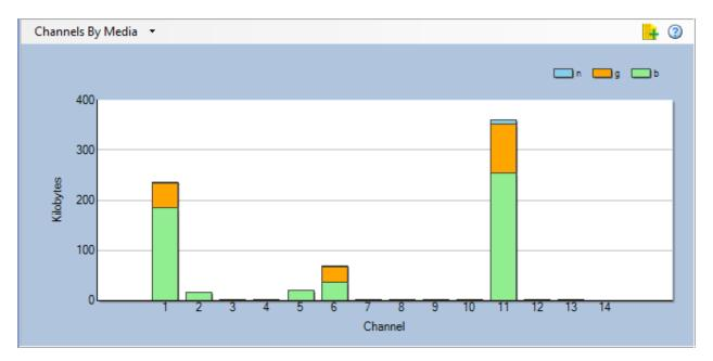
Each bar in the Channels by Media graph represents the total amount of data in kilobytes that has been transmitted on a channel. Wi-Fi traffic is categorized by the type of 802.11 media being used.
