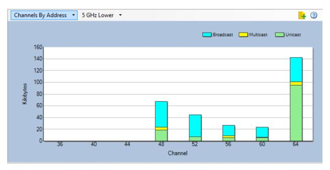
The traffic is broken down into three categories, each represented by a unique color:
