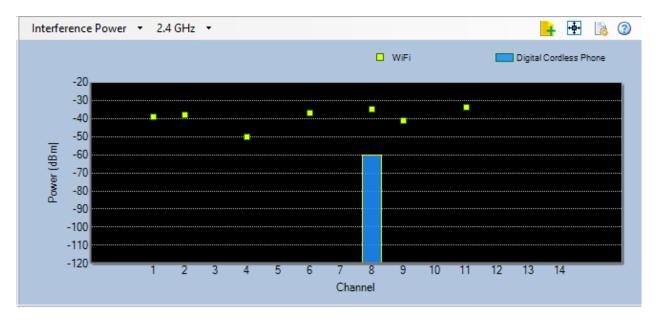
As noted in the color legend above the main portion of the chart, the yellow points on the graph represent the current signal strength of the strongest AP detected on each channel; hovering over the point provides the device's name and MAC address. The point's location on the chart indicates the level of interference that it is experiencing; as the interference level climbs, the device's performance can suffer as a result.
