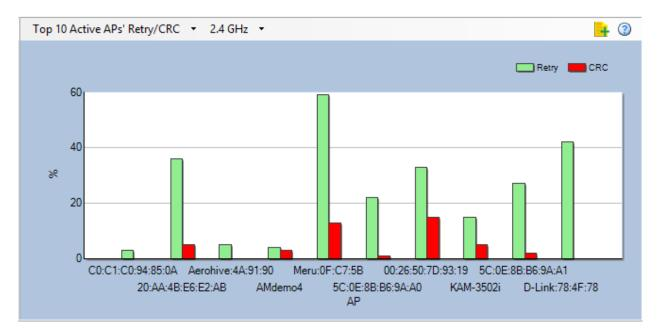
As shown above, the CRC and Retry packets are color-coded, with red for CRC and green for Retry. The APs are identified by name, IP address, or whatever identification is used on the network. If you place the cursor on an AP, a tooltip will pop up showing the following basic information about the AP, in addition to the percentages of Retry and CRC packets transmitted by the AP:
