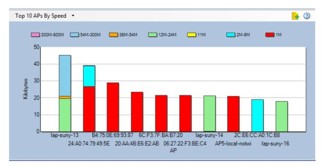
Each bar in the Top 10 APs by Speed graph represents the volume of data transmission being recorded involving a specific AP. It also provides a breakdown of the transmission by
