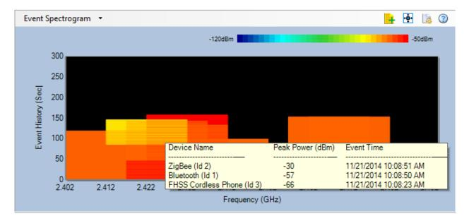
**Note:** If you place the cursor over the line/band, a tooltip will pop up showing some basic information about that device, such as the type of the device, its peak power, and the time of it being detected.
