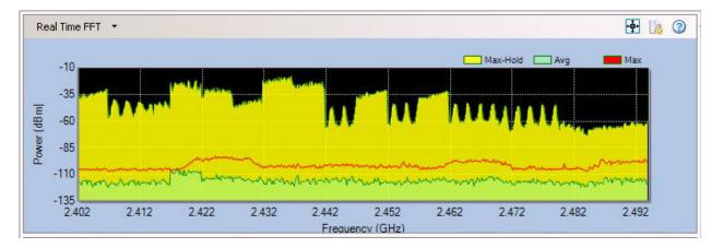
The figure below shows the RF spectrum pattern of a Bluetooth iPhone.
