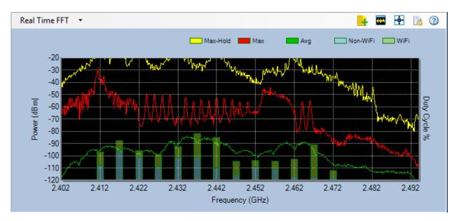
FFT Graph Showing Channel Duty Cycle
