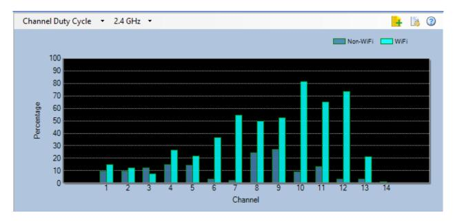
**Note:** If you place the cursor over a channel, a tooltip will pop up showing the Maximum and Current power readings on that channel.
