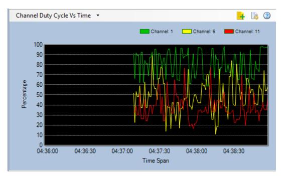
As shown above, the graph will display up to three channels at a time in color-coded lines. The channels can be modified via the chart configuration, as explained below.
