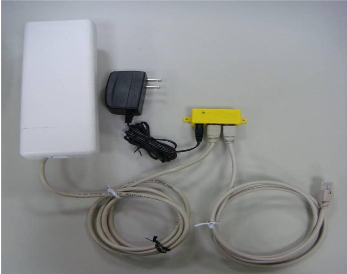
**Notes:** Use **Reset button** on POE injector. Push continually the reset button of POE injector about 5 ~ 10 seconds to reset the configuration parameters to factory defaults.
